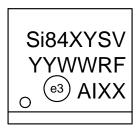
Figure 17. Isolator Top Marking
